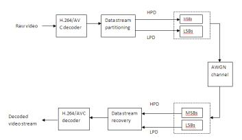
Fig 3. Block diagram of the proposed UEP scheme
