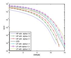
Fig2SERversus SNR for a range of alpha values for 16HQAM
