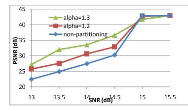
Fig 5 PSNR performance the UEP scheme for the Suzie video sequence
