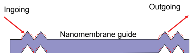
Fig. 4. 3D-sculpted nanomembrane coupling configuration using pyramidal (or, alternatively, hemispherical, shown as dotted red lines) spatial patterns
