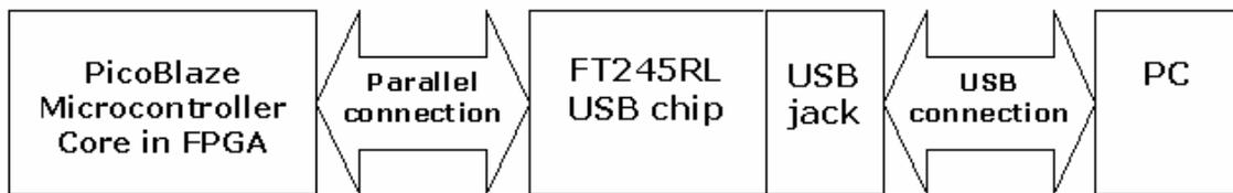
Fig. 4. proposed block diagram for Microcontroller with USB
