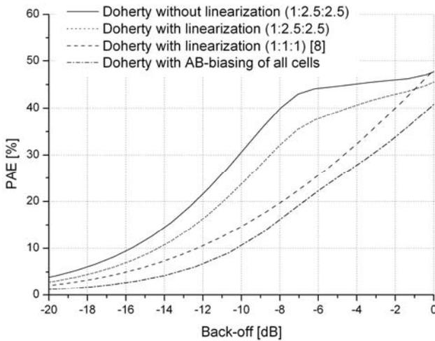
Fig. 2. Power added efficiency of three-way Doherty amplifier for device size ratio 1:2.5:2.5
