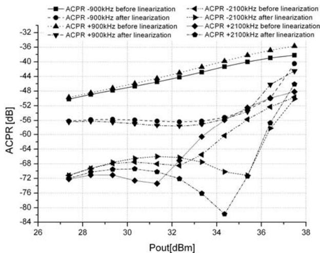
Fig. 5. ACPR before and after linearization of three-way Doherty amplifier for a power range at  $\pm 900\text{kHz}$  and  $\pm 2100\text{kHz}$  offsets from carrier frequency
