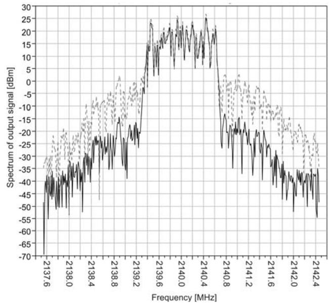
Fig. 4. Simulated spectrum of the output voltage for three-way Doherty amplifier for device size ratio 1:2.5:2.5 for OQPSK digitally modulated signal before (dashed line) and after linearization (solid line) for 35dBm output power
