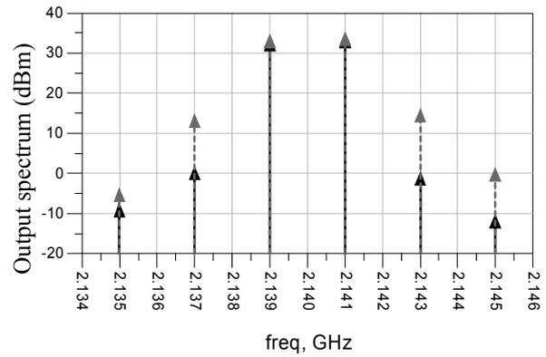
Fig. 3. Output spectra of three-way Doherty amplifier for device size ratio 1:2.5:2.5 for 33dBm average output power of fundamental signals; before (dashed line) and after the linearization (solid line) in case of 2MHz signal space
