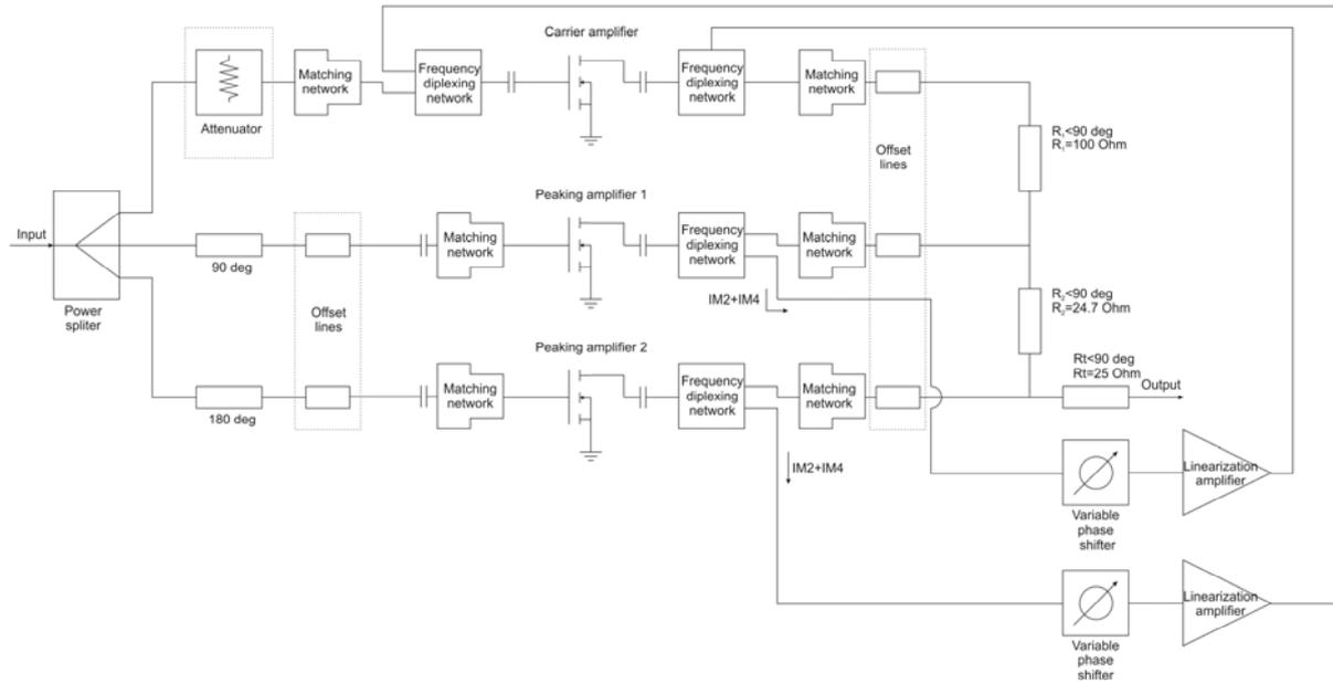
Fig. 1. Three-way Doherty amplifier with additional circuit for linearization
