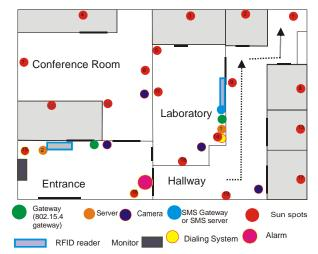
Fig. 1. Scheme of WSN and RFID implementation plan at the FEEIT's premises.
