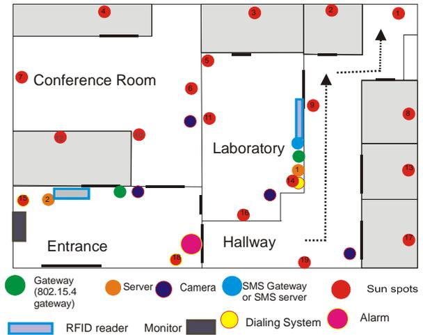
Fig. 1. Scheme of WSN and RFID implementation plan at the FEEIT's premises.
