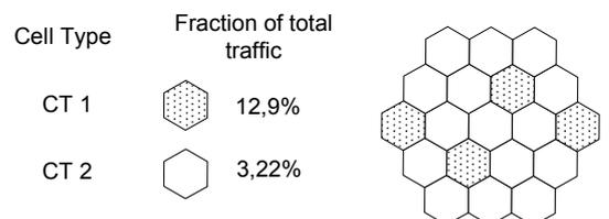
Fig. 3: Simulation model.
