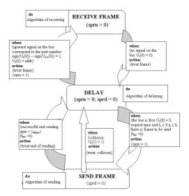
Fig. 3. State algorithm chart of object Host
